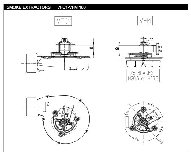
Used in a wide range of products such as, pellet stoves, pellet boilers, Standard for all motor types 230V-50Hz: insulation class H; thermal protector, with /without housing. available with/without hall sensor for motor H25
